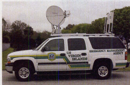
2. Portable satcom earth-station terminals such as this provide flexibility for mobile broadcast and SNG applications.
